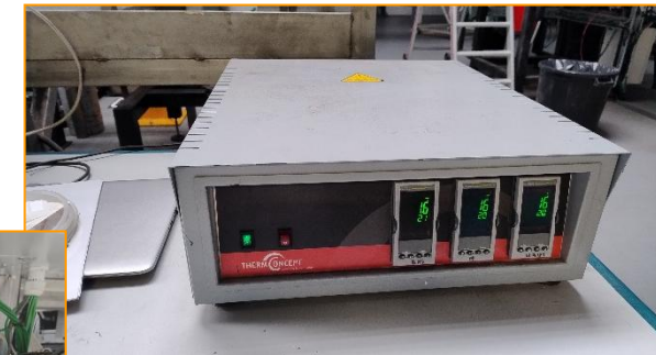
The 3 PID for the heating control unit
