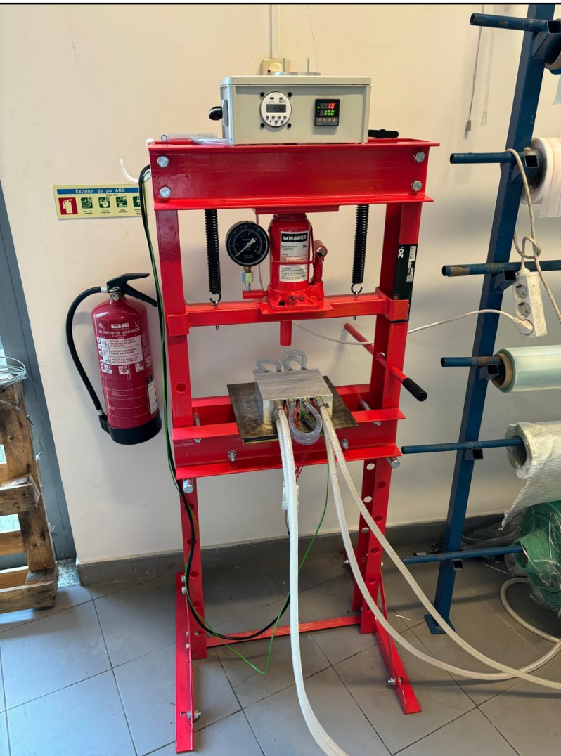
Hydraulic press developed to produce a chestnut-based candle holder
